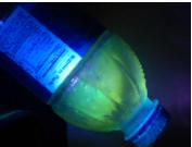
**Fuming Orange** is also incredible versatile and works with almost any light source currently in your laboratory. Whether you work with: UV inspection lights, high power NDT lamps, lasers, UV penlights or even UV led lights, when excited anywhere from 365 nm to 530 nm, **Fuming Orange** will glow revealing the print. Colored band-pass filters or glasses will intensify the effect.
